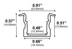
Type:.....LED Channel Material:...Aluminum 6063-T5 Surface:....Clear Anodized Height:.....14.50mm / 0.57" Width:.....23.00mm / 0.91"
