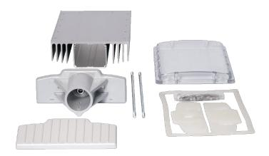
The **905 Series Street** is offered as **all-inclusive finished product** with Heatsink Extrusion, Special design Aluminum Side Covers with Gaskets, Polycarbonate Front Window with Sealing Gasket, Mounting Brackets and Hardware. **Street Light** Set includes side covers that is compatible with **street light poles 45mm in diameter**.
