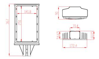
Heatsink Extrusion 6063-T5 Clear Anodized Aluminum
