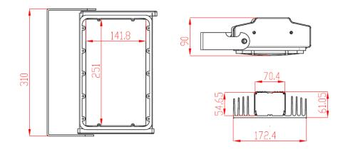
Heatsink Extrusion 6063-T5 Clear Anodized Aluminum
